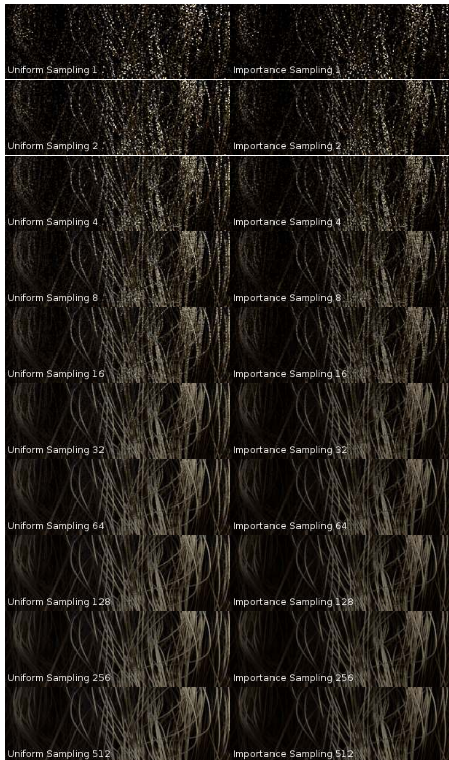
Figure 6.6: Comparison of the image quality between uniform sampling and importance sampling for various pixels per sample, indicated in the bottom left corner. As the pixels per sample increase, the noise of the image becomes smaller.
